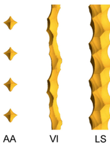
Figure 13. Crystal pore topography of the studied dipeptides as determined with a 2.6 Å probe. Reprinted with permission from Afonso et al. [33] Copyright 2010 John Wiley & Sons, Inc.
