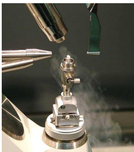
Figure 14. Photograph of the high pressure X-ray data collection apparatus. The crystal is mounted in a capillary and attached to a miniature valve.
